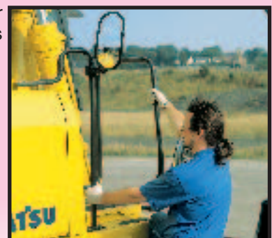
Large handrail for safe access
