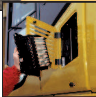
Easy cleaning of air conditioner filter Easy removal/installation of air conditioner filter element, without tools facilitates easier cleaning.
